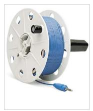
50m measurement cable coilded around a metal drum. Connection to one end of the cable is accomplished with a jack which is integrated into the drum. The other end is equipped with a banana plug. The drum axle with handle can be removed for space saving storage.
